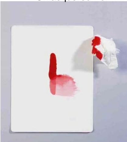
A penetrative dye is painted onto samples of unlacquered and lacquered liner and left for 10 minutes. When it is wiped off the results show that the dye has been absorbed by the unlacquered liner while the lacquer has prevented any absorption in the other sample. This level of protection means that Alkorplan membranes are better protected than products without this level of protection.
